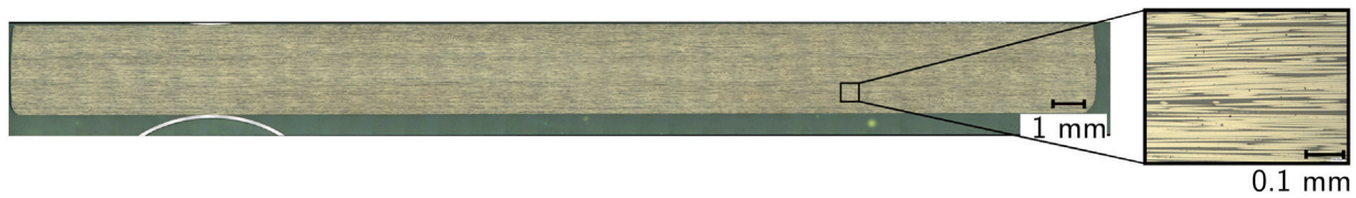
Fig. 1. Micrograph (cross section parallel to the fibers main axis) of the consolidated samples before deconsolidation tests. The initial porosity content is not measurable.
