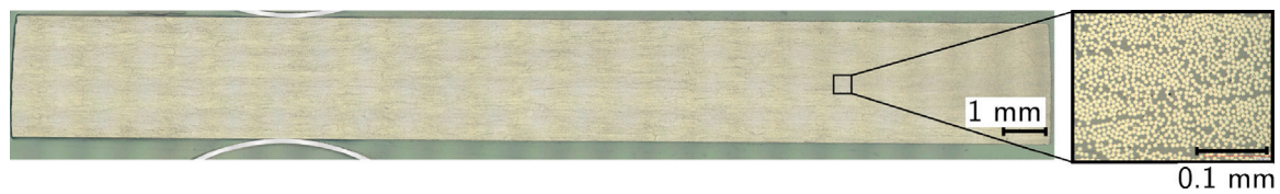
Fig. 5. Micrograph of the consolidated samples before deconsolidation tests. The initial porosity content is not measurable.
