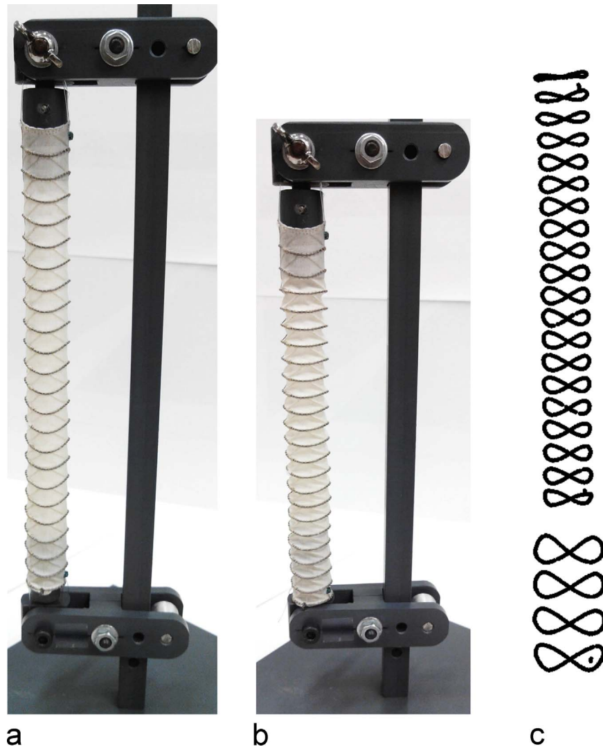
Fig. 4 – Experimental setup inserted in the microtomograph to derive the geometry of SG modules in stretched (A) and tension-free (B) states. Example of stent neutral axes extracted from microtomography scan images (C).
